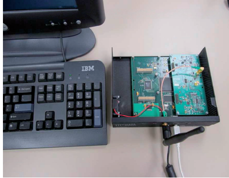
Figure 4. The testbed wireless station setup.
